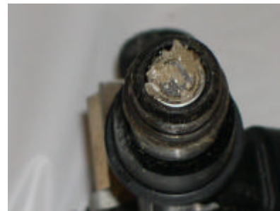
Caramelised and gummy deposits on injectors – 2001 Pontiac Venture
