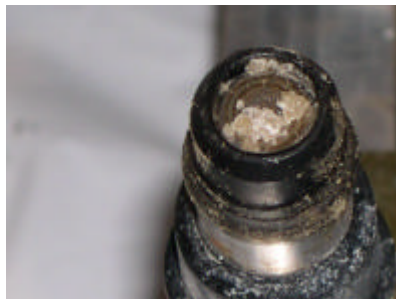
Caramelised and gummy deposits on injectors – 2001 Pontiac Venture
