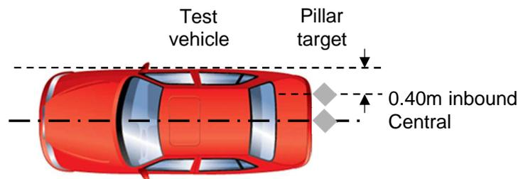
**Figure 9 - Reversing car-to-pillar central and 0.40m inbound at impact position**
