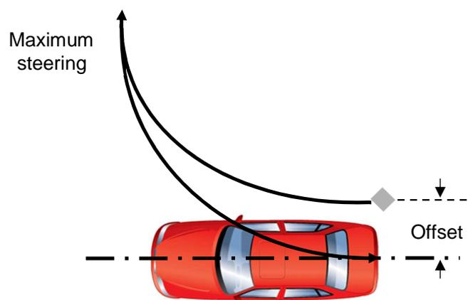
Figure 7 - Offset determination method (effect exaggerated)
