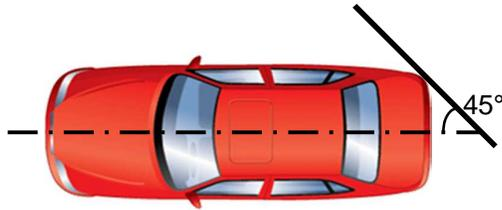
**Figure 5 – Identifying the rear corner of the test vehicle**
