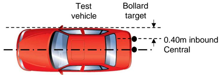
**Figure 8 – Reversing car-to-bollard central and 0.40m inbound at impact position**
