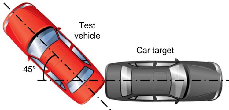
**Figure 4 – Reversing car-to-car 45° centre at impact position**
