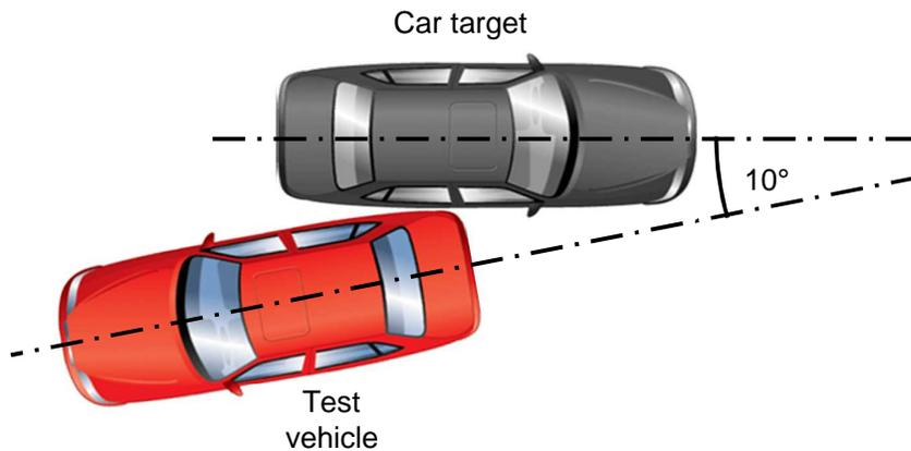
**Figure 6 – Reversing car-to-car 10° side at impact position**
