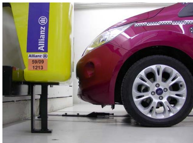
In order to fulfill the test criteria for pedestrian protection (lower leg to bumper), almost every manufacturer integrates a so-called lower stiffener as part of the front bumper concept. Assembled in spoiler height, the test dummy equipment receives an additional impulse, which prevents an excessive angle of bending in the knee area. Is the lower stiffener integrated in
