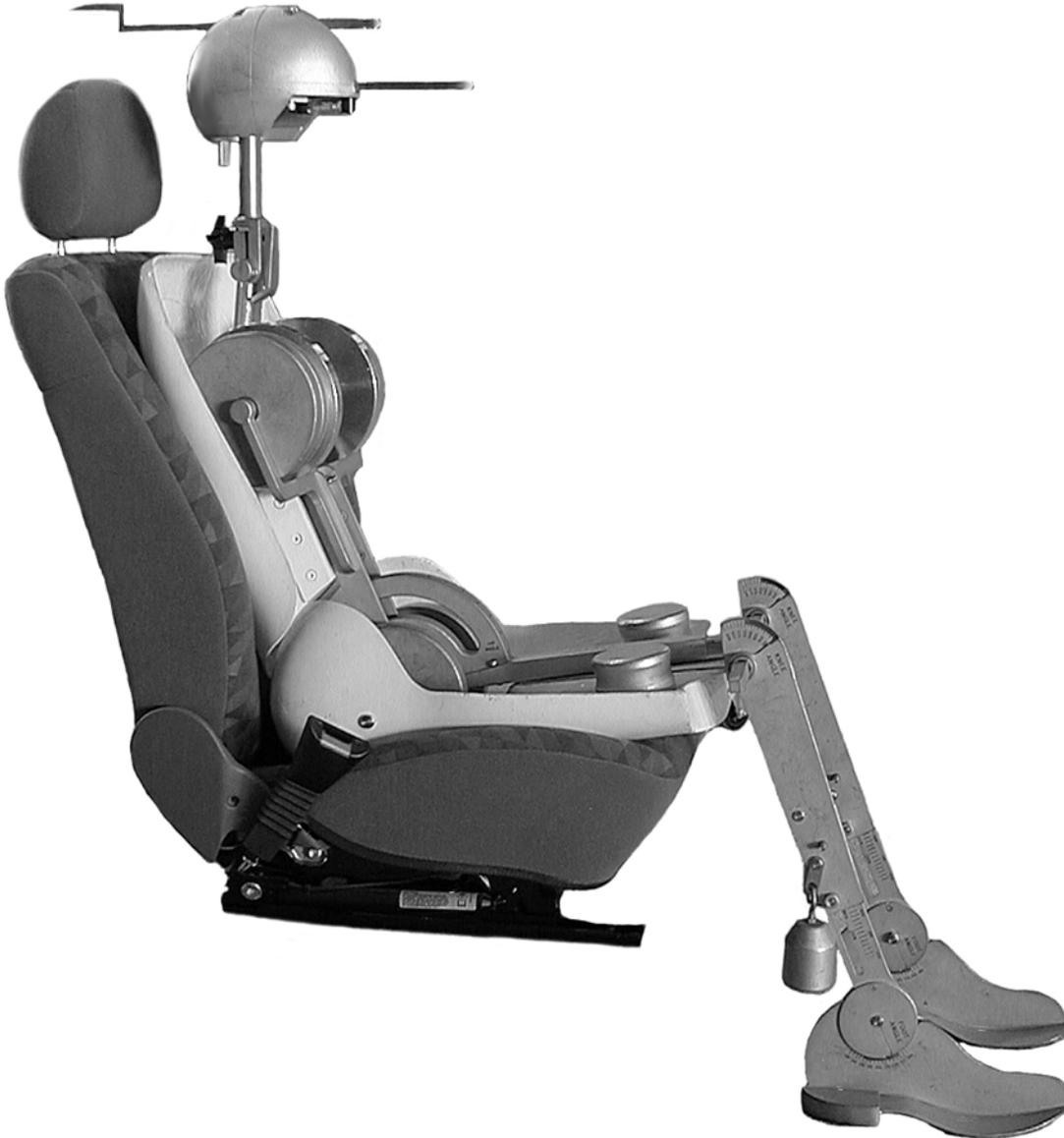
**Head Restraint Height Measurement**
