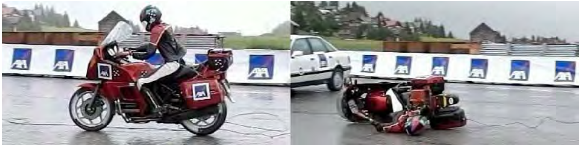
Picture 3: Both motorcycles at t=1s. With ABS controlled braking (left), without ABS (right).
