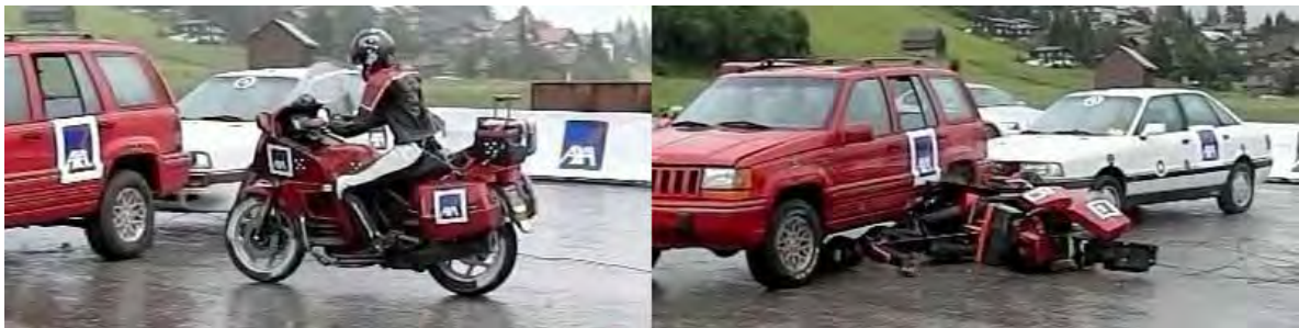
Picture 4: Both motorcycles at t=1.5s. With ABS (left) still braking, without ABS (right) already crashed into the car.
