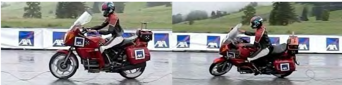
Picture 2: Both motorcycles at t=0.5s , braking. On the right part of the picture: motorcycle without ABS falling.
