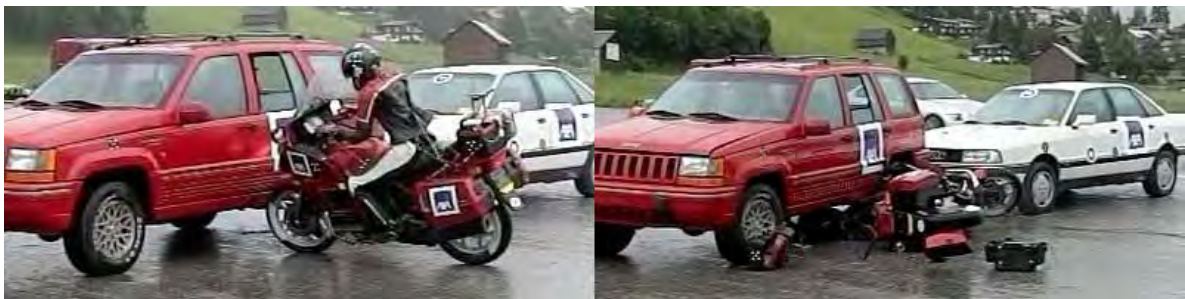
Picture 5: Both motorcycles at t=2.0s. With ABS (left) the motorcycle was able to stop in front of the car.
