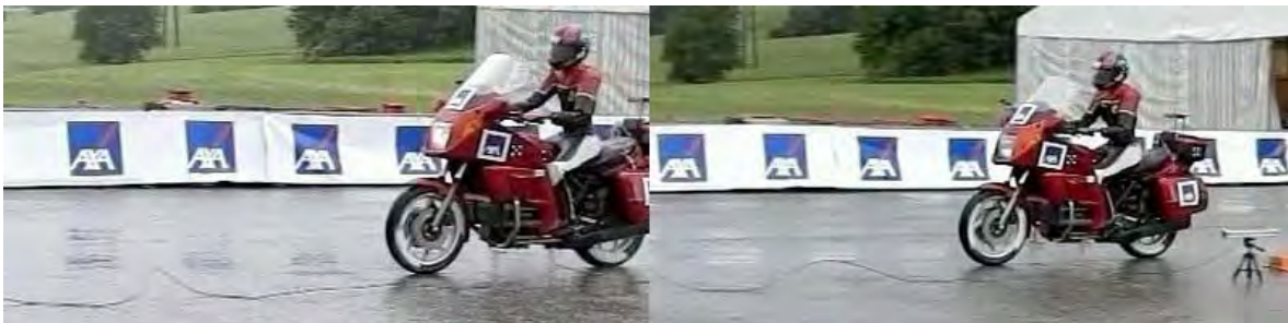
Picture 1: Both motorcycles at t=0s with a velocity of 50 km/h, starting to brake
