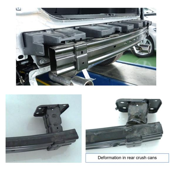
**Note:** The design and the material of the bumper reinforcement produces a good deformation that absorbs the energy of the crash.
