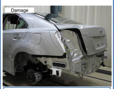
The quarter panel and rear side member were damaged and needed to be repaired.
