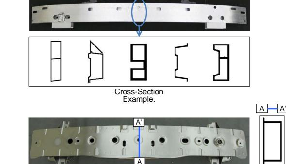
Example of a cross-section of high-strength reinforcement.
