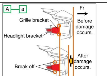
Example of a structure where the mating section of the radiator grille and headlight break off to prevent damage from spreading to the headlight.
