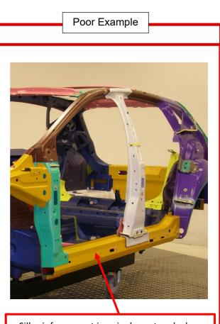
Sill reinforcement is a single part and when damaged will require sill cover removal and sectioning.
