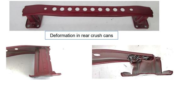
**Note:** The design and the material of the bumper reinforcement produces a good deformation that absorbs the energy of the crash.
