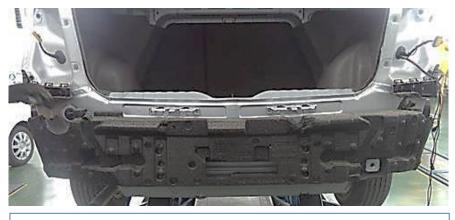
Only polystyrene mounted on the rear panel
