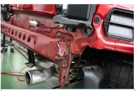
Deformation in bumper reinforcement
