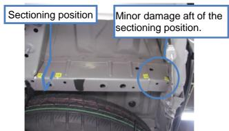
Example of a structure that allows damage to end aft of the sectioning position of the rear side member.
