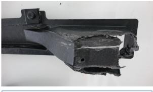
The bumper reinforcement was broken
