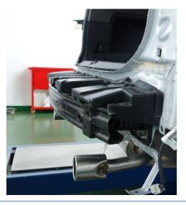
Deformation in bumper reinforcement
