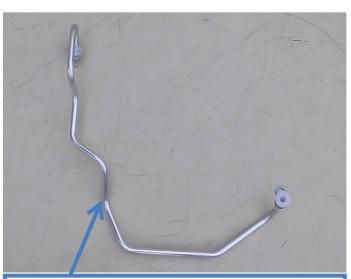
Repair was done just replacing the front pipe.
