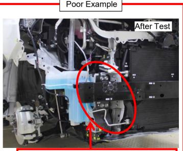
Front section of the pipe was damaged.
