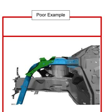
Intrusive requirement to remove A Pillar outer section
