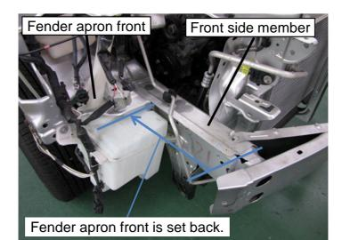
Example of a structure where the fender apron front is set back from the side member.
