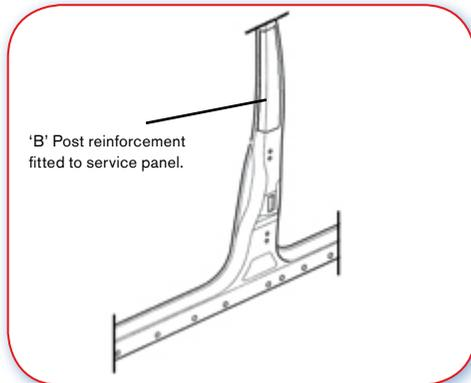
13.2.E Good example. 'B' Post with a UHSS reinforcement can be sectioned.
