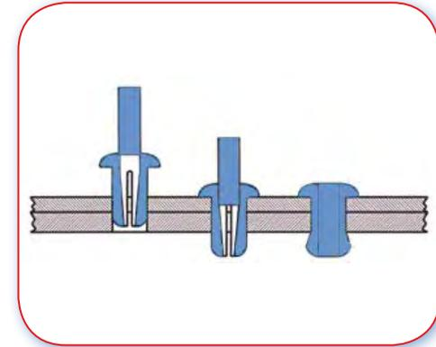
C.10.1 An example of poor clips. Pin will be lost on removal.
