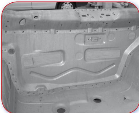
Poor Example. Rear centre panel with the flange pointing upwards hinders drilling, and more importantly, resistance spot welding operations
