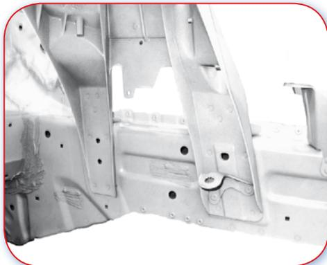
5.3.C Good example. Showing a separate suspension strut tower fitted to the front chassis leg. The front panel reinforcement is only supported by a bracket attached to the firewall.
