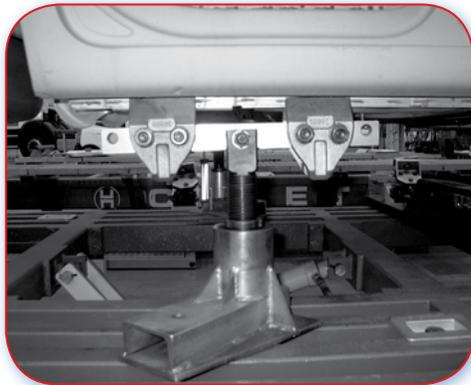
Good Example. Sill panel with a classic longitudinal flange facilitates the use of a universal anchoring system.
