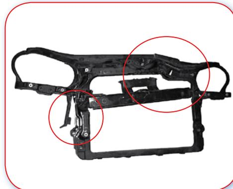
7.2.B Good example. On impact, the panel has broken, allowing parts fitted to the panel to move, but not to be damaged.
