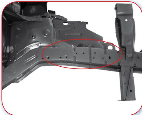
9.2.A Poor example. Chassis leg with too many reinforcements, leaving no area for any proper section.
