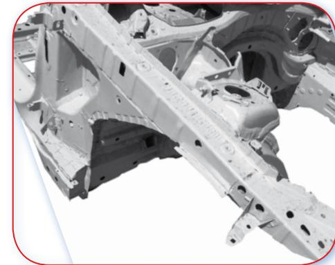
6.0.C Typical examples of front panel reinforcements.
