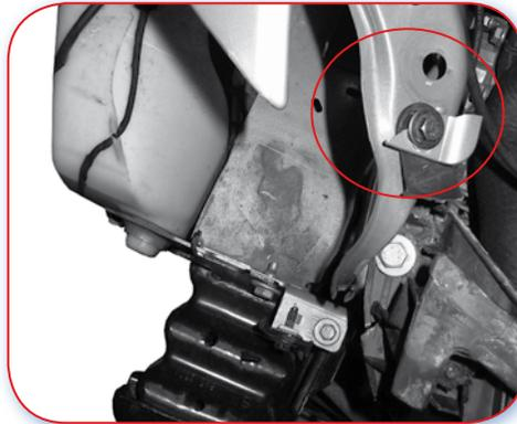
7.2.E Good example. On impact the panel has broken, allowing parts fitted to the panel to move but not to be damaged.
