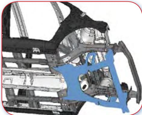
10.0.C Good example. Sub-frame as a two piece unit. Separable in the middle.
