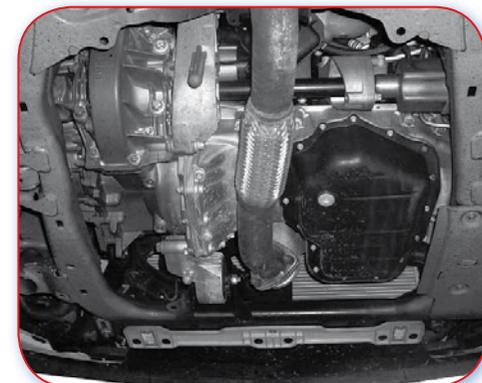
10.0.E Poor example. Single round sub-frame, any damage means complete replacement will be required.
