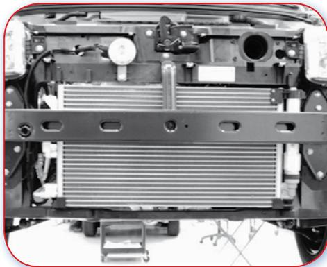
7.2.G Good example. The front panel comprises a landing panel but no lower parts. Costly parts set back enough to reduce damage.
