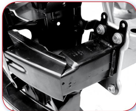
3.0.K Good example. A bolt-on crush can. This is an average length crush can made from steel.
