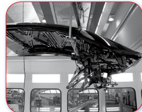
15.2.B Good example. Appropriate lifting tool reduces the number of people required and reduces risk of damage.
