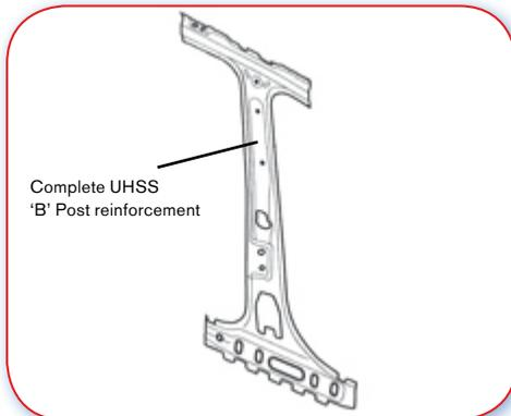
A.2.1 Poor example. 'B' Post made out of UHSS, requires complete replacement.
