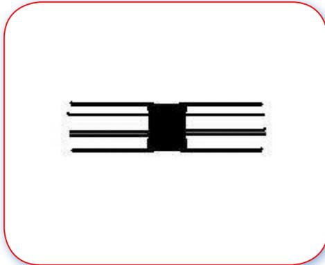
B.4.1 Step one: Spot weld in multilayered stack.
