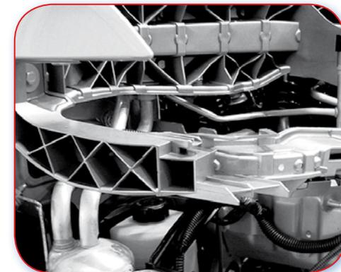
7.2.K Good example. Auxiliary parts are fitted further back (apart from the horn). They are made out of plastic, so no paint is necessary.
