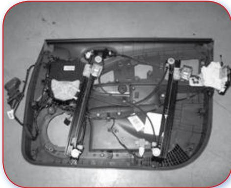
Good Example. Most of the door mechanisms are fixed directly into its trim, which will facilitate repair and replacement operations.
