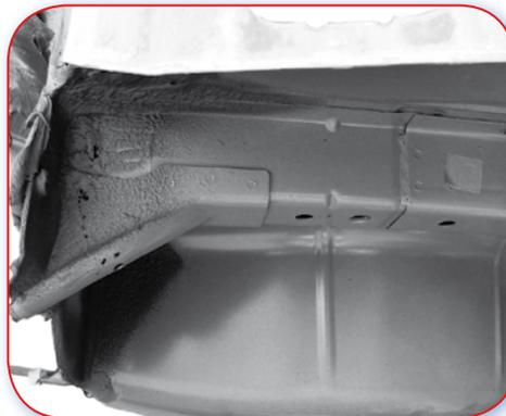
20.1.A Good example. Chassis leg is sectionable on a natural joint. This will improve ease of repair.
