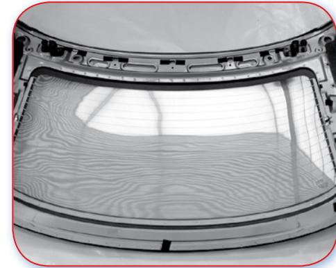
15.8.A Poor example. Glass panel bonded into complex shaped folding roof panel.
