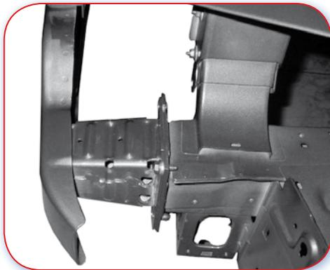
3.0.H Good example. A bolt-on crush can. This is an average length crush can made from steel.
