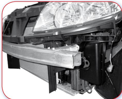
2.1.D Poor example. Narrow reinforcement. No pedestrian protection bar. Good distance between reinforcement and cooling pack. No parts clip onto reinforcement.
