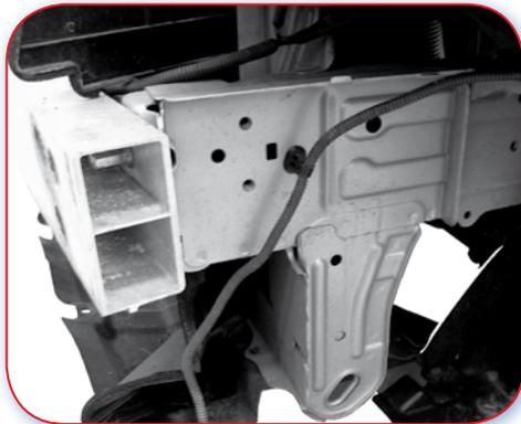
3.0.C Poor example. No crush can, so the chassis leg will be damaged on impact.
