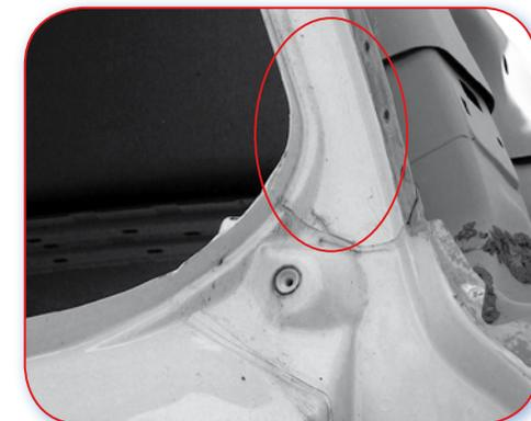
17.2.E Good example. The drain channel is made out of one piece, joining the outer and inner panel.
