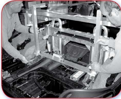
15.5.A Good example. Substantial jigs to check alignment of critical locations.
