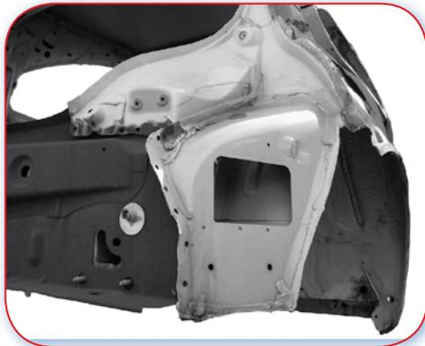
17.1.C Good example. The rear outer panel and rear panel are separately joined by the light panel and bridging panel, ending in outward facing flange joints.
