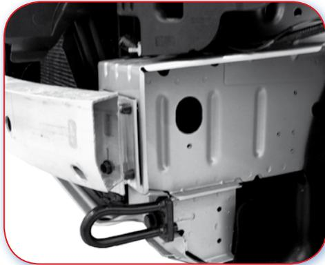
3.0.B Poor example. No crush can, so the chassis leg will be damaged on impact.
