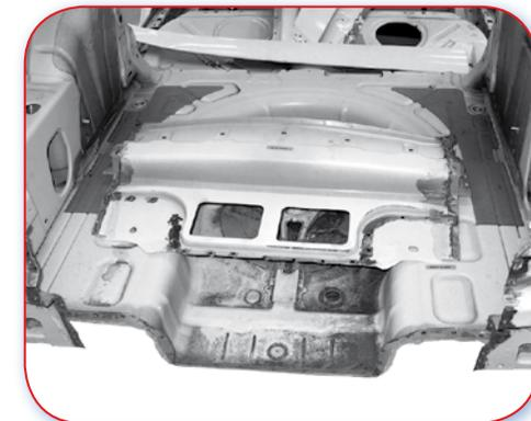
18.1.F Good example. As the rear panel is fitted last, removal of the rear panel will not require any other panel to be removed.
