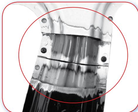
13.2.H 'B' Post can be sectioned through reinforcements and both outer and closing panel without having to cut into upper roof rail. Most reinforcements made from UHSS cannot be sectioned.
