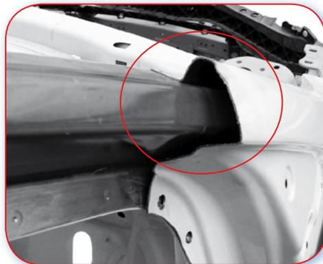
12.0.D Good example. 'A' Post outer panel set away from reinforcement, which will avoid damage on sectioning.
