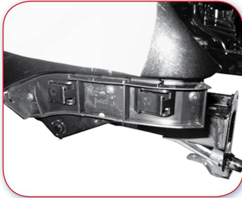
1.1.B Good example. Bracket is supporting the panel and bumper independently.
