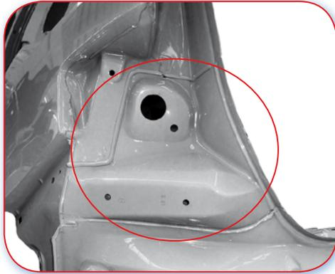
17.1.A Good example. The rear outer panel and the rear panel are joined separately, bridged by the light panel and bridging panel.
