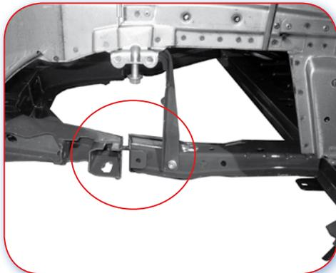
10.0.B Good example. Sub-frame can be separated to remove damaged front part.
