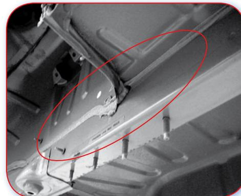
20.3.C Poor example. Chassis leg is sandwiched between the wheel arch and boot floor, which is difficult to remove and replace.
