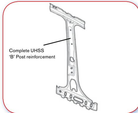
13.2.A Poor example. 'B' Post made out of UHSS, requires complete replacement.
