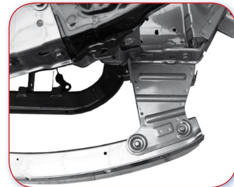
3.0.L Good example. A bolt-on crush can. This is an average length crush can made from steel.
