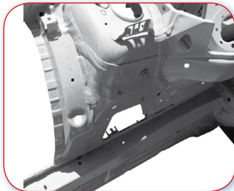
4.1.H Good example. No inner wing, just a reinforcement joining the panel reinforcement and chassis leg. An arch lining forms the joint between the front panel, inner wing and panel reinforcement.
