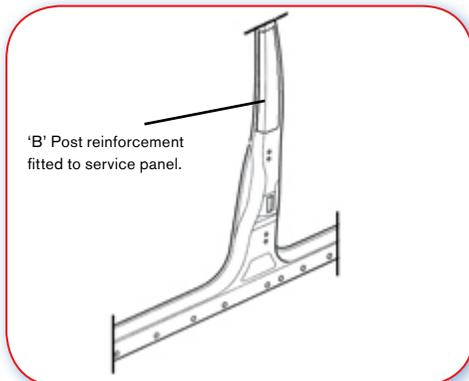
A.2.2 Good example. 'B' Post with a UHSS reinforcement can be sectioned.
