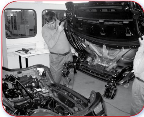
15.1.B Poor example. Removal of the complete roof in stowed position is difficult due to the shape and limited space available.
