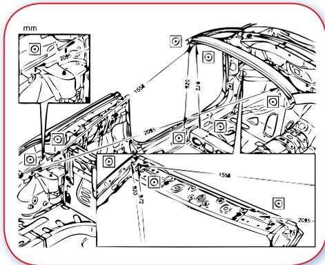
15.6.A Good example. Reference dimensions to check alignment of critical locations.
