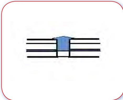
B.4.3 Step three: New panels joined with plug weld.
