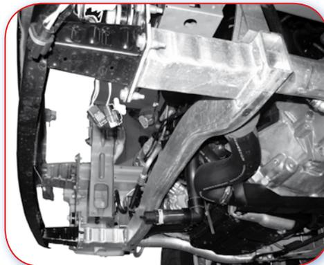
10.0.D Good example. Sub-frame segmented, any damaged parts can be easily replaced.
