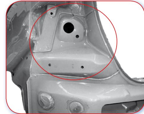
17.2.C Good example. The rear outer panel and rear panel are joined separately, bridged by the light panel and bridging panel.
