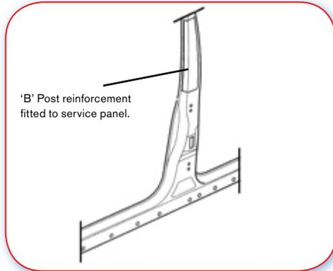
13.0.A Good example. 'B' Post with a UHSS reinforcement can be sectioned.
