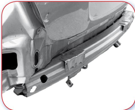
22.0.B Beam has been pushed into the rear of the car and has deformed the rear inner and the outer panels, pushing the outer panel into the rear door.
