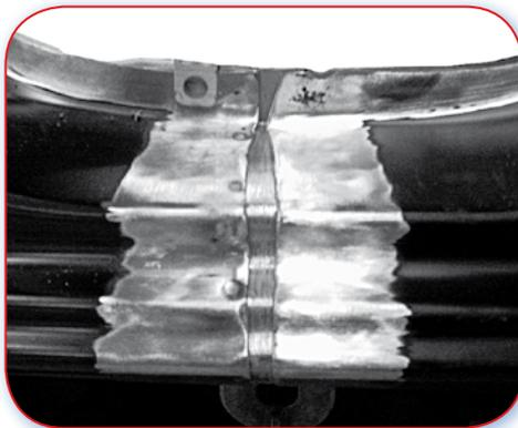
16.1.K Poor example. The alignment and joining of the supplied service panels do not match.
