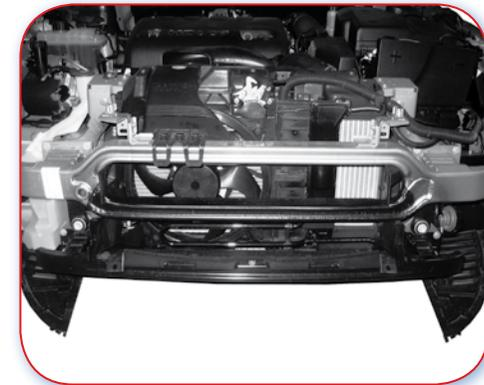
2.1.B Good example. Parts clip onto the bumper beam for easy release.
