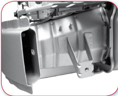
3.0.I Good example. A bolt-on crush can. This is an average length crush can made from steel.
