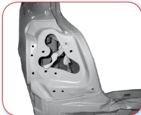
17.2.A Poor example. Rear quarters built up from several parts cause difficulty when separating and aligning parts in repair.
