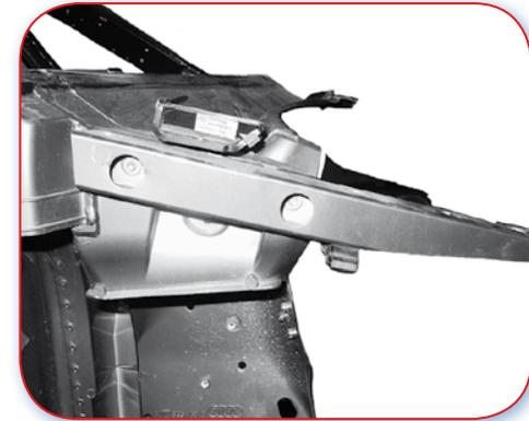
12.1.C Good example. Side panel reinforcement bolted onto plenum chamber/'A' Post. This will ease the replacement.
