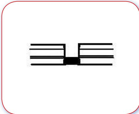
B.4.2 Step two: Spot weld removed to allow removal of outer panels.
