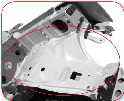
4.1.B Poor example. Both pictures show an inner wing that extends to the front panel and light fittings. This does not allow movement of parts on impact and results in them being damaged.
