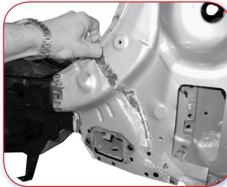
18.1.B Poor example. The rear panel has been fitted behind two panels which need removing before it can be replaced.
