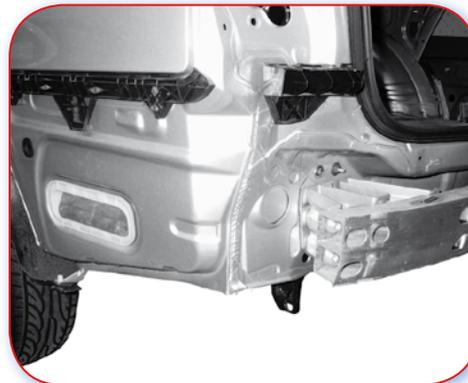
21.0.D A bumper beam fitted on crush cans, which absorbs energy on impact and creates space for deformation.
