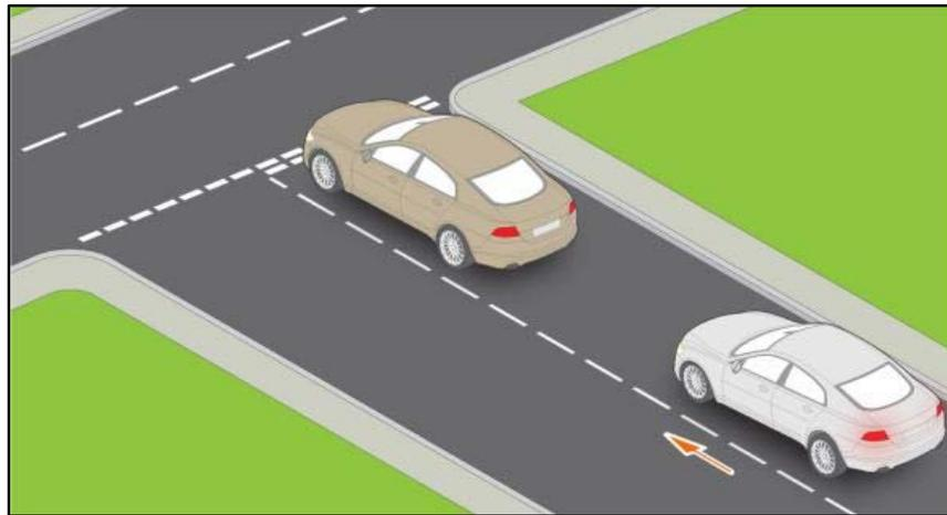
Figure 2 – Car-to-car front-to-rear collision test scenario
