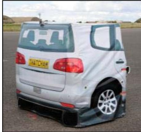
Figure 1 – Euro NCAP Vehicle Target (EVT)
