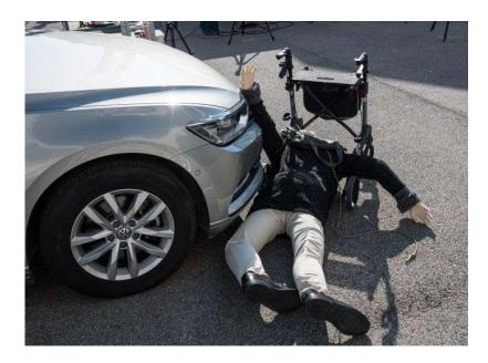
AZT impact tests with a CTS biofidel pedestrian dummy (representing a female, 70 kg, 163 cm) run with 3, 6 and 20 km/h forward and 3 km/h reverse. The outcome shown here, was the result of a 3 km/h forward touching of the rollator only that made the senior fall along the car front, injuring hershoulder, cutting her face in the rollator and finalizing in a hard head impact at the bottom
