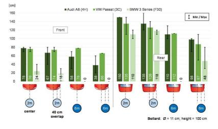
(a) Comparison of position and orientation for bollard
