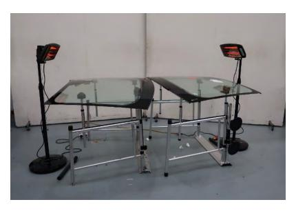
Image: Windscreen controlled heating arrangement
