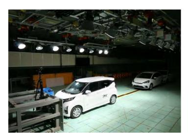
With the new lighting system, lightings can be divided into two parts, front and rear. Therefore, in the multiple crash test, sufficient illumination can be provided to the second (crashing) vehicle.
