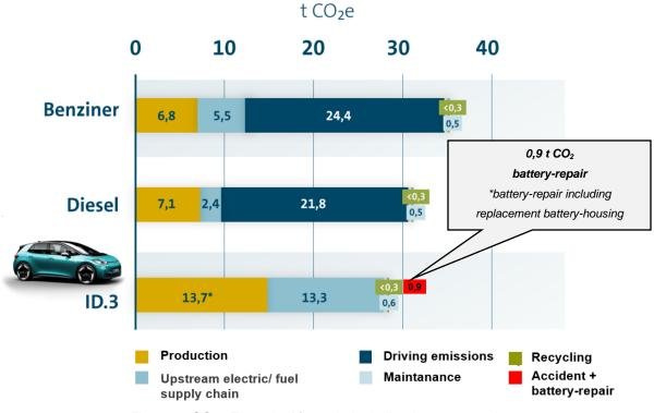
Figure 3: CO-2 Footprint life cycle including battereyrepair
