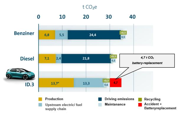
Figure 2: CO-2 Footprint life cycle including batteryreplacement
