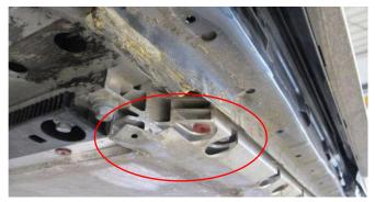
Figure 1: Damaged battery housing
