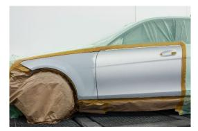
Example of a vehicle with repaired fender and refinish painting with color matching of the adjacent component in the same level (driver's door).
