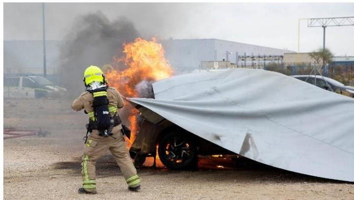
Fig. 1.- Fire blanket to extinguish fire on the tested electric vehicle.
