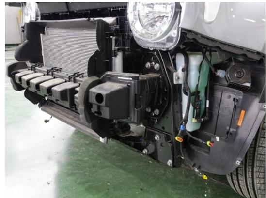
To demonstrate, we compared two models of vehicle of the same brand which is one of the most important in the Colombian market, with a representative sales of 18%. These two vehicle models are similar because the latest in the model evolution of the first, but the latest model has less elements to reduce energy of the crash, like front bumper reinforcement and front crush cans in the front structure. The table show the differences between these two models and the results.
