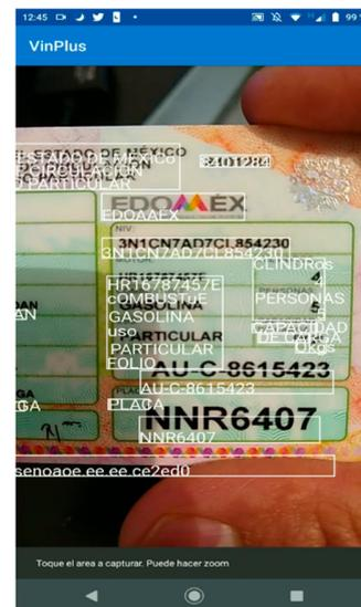
With images from a VIN sticker or the car registration, the VINPlus App can read the 17 characters of the identification series. By innovating with text recognition technologies through images, the work of VINPlus users is easier than ever.
