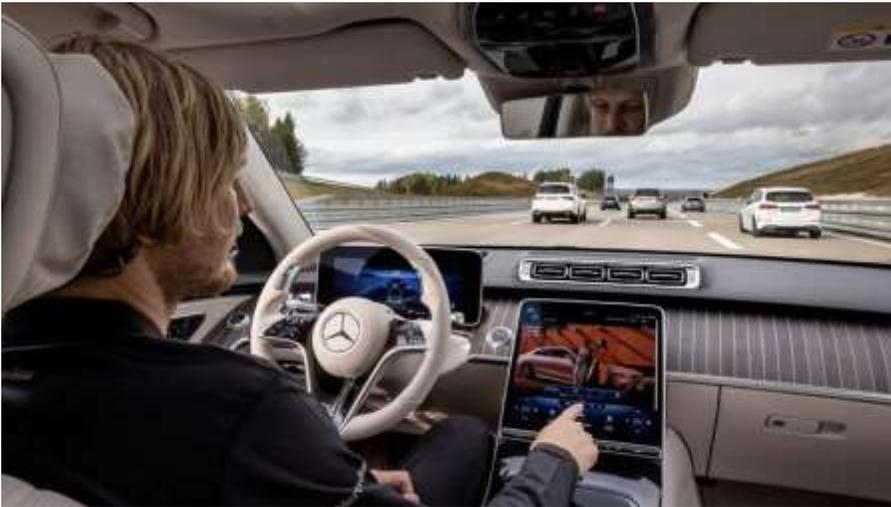
ALKS is designed to operate only on divided highways under certain conditions at speeds of up to 60 km/h. However, suggested amendments at the UN are already proposing 130 km/h running. These systems also only allow the car to be guided in-lane and cannot automatically steer out of lane. ALKS allows the driver to undertake secondary tasks through the on-board infotainment system. E.g. emails or movies.
